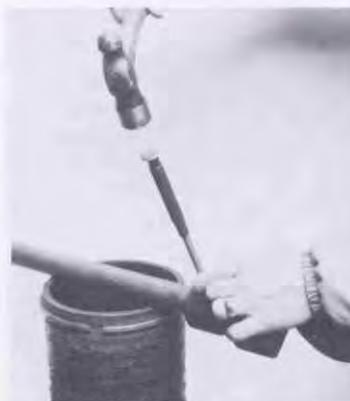
**4** Drive out pin (34) and remove broken piece of coupling (35) from upper stem. Remove nut (32) and bolt (31). Pull broken coupling from lower stem.
