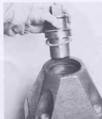
**11** Screw operating nut (1) onto upper stem with lower Delrin bearing (42) in place. Install remaining Delrin bearing (42) between two races (5) on operating nut.
