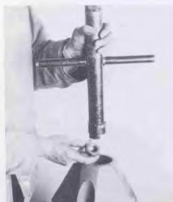
**10** Thread hex stop nut (12) onto upper stem and tighten securely with combination tool.
